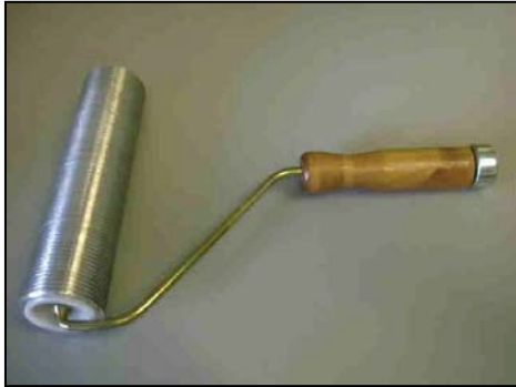
Fig. 5 – A laminating roller can make installations onto high temperature surfaces much easier. This tool can also be used on large flat surfaces where Stricture Banding™ cannot be effective.
